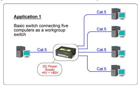
The following figure illustrates a basic switch model connects four computers via Cat.5 cables and uplink to a fiber backbone network.
