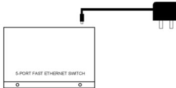
2. Connect the power adapter cable to the switch before connecting the adapter to the AC outlet.
