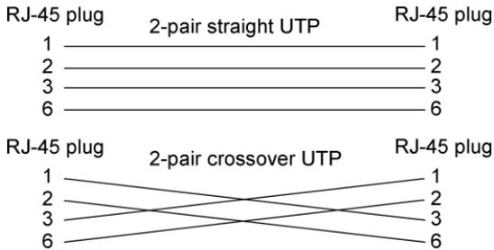
It is suggested to use straight-through UTP cables for all UTP connections. The maximum length and UTP cable categories used for the connections to a 10BASE-T device and 100BASE-TX device are:
