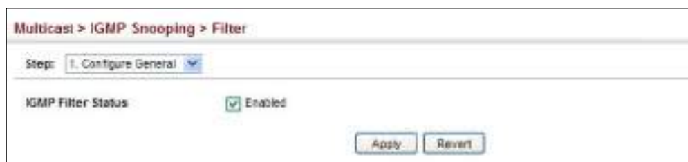
Figure 389: Enabling IGMP Filtering and Throttling
