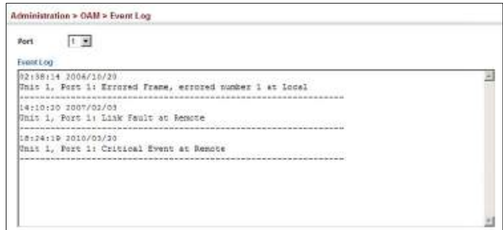
Figure 361: Displaying the OAM Event Log
