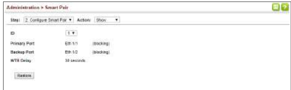
Figure 373: Displaying Port Members of a Smart Pair
