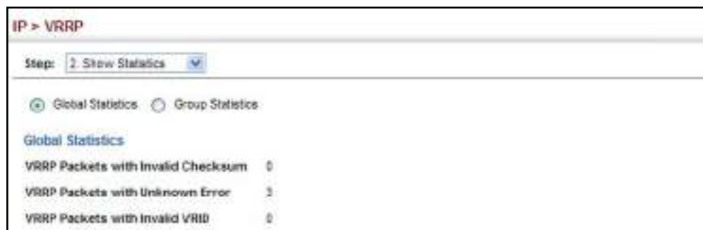
Figure 520: Showing Counters for Errors Found in VRRP Packets
