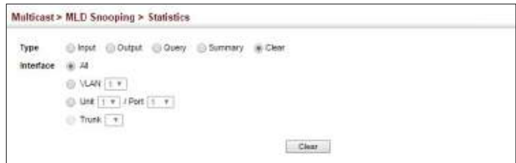
Figure 410: Clearing MLD Snooping Statistics
