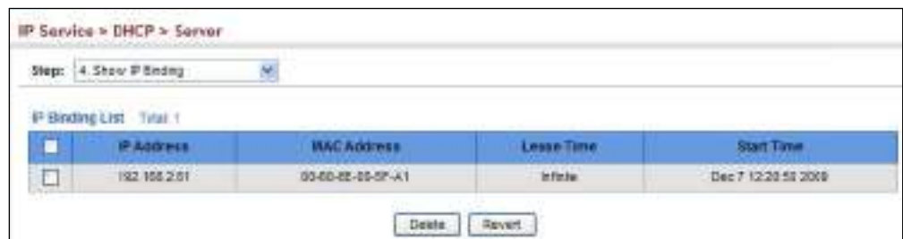
Figure 499: Shows Addresses Assigned by the DHCP Server
