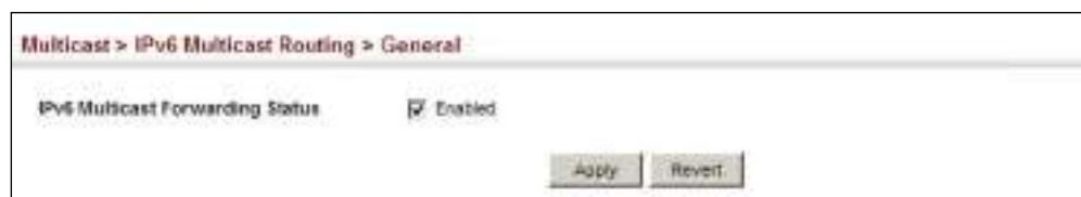
Figure 568: Enabling IPv6 Multicast Routing
