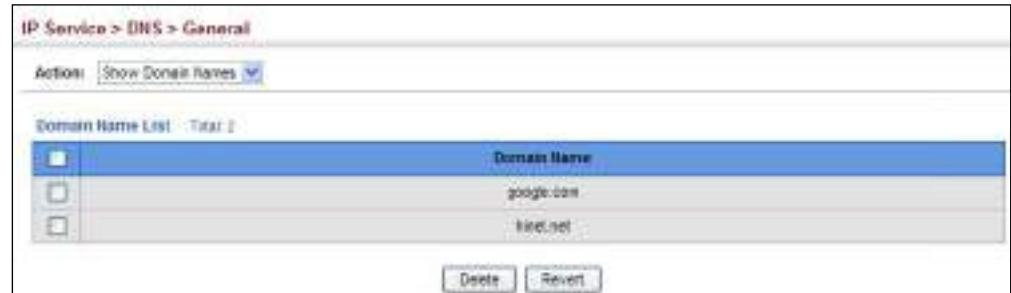
Figure 480: Showing the List of Domain Names for DNS
