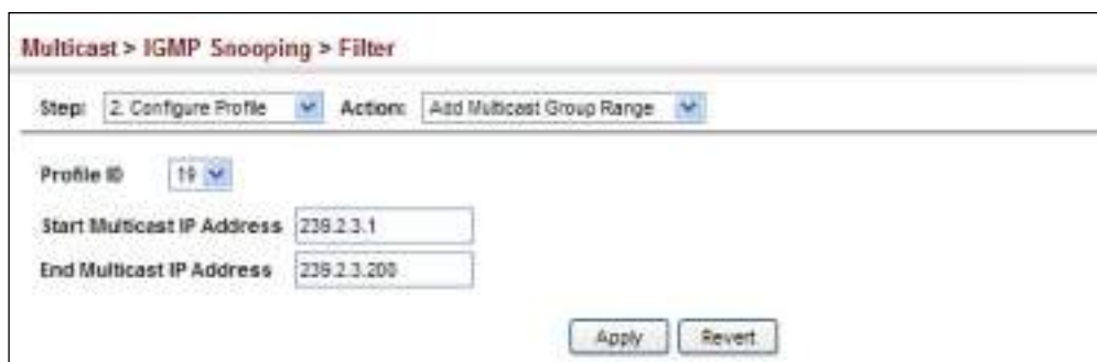
Figure 392: Adding Multicast Groups to an IGMP Filtering Profile
