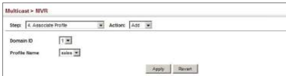
Figure 427: Assigning an MVR Group Address Profile to a Domain
