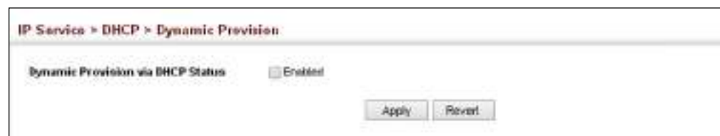
Figure 491: Enabling Dynamic Provisioning via DHCP
