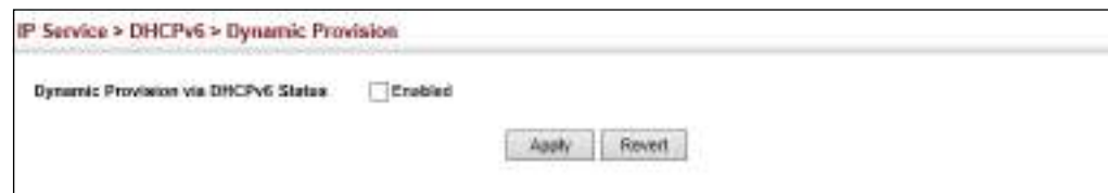
Figure 503: Enabling Dynamic Provisioning via DHCPv6
