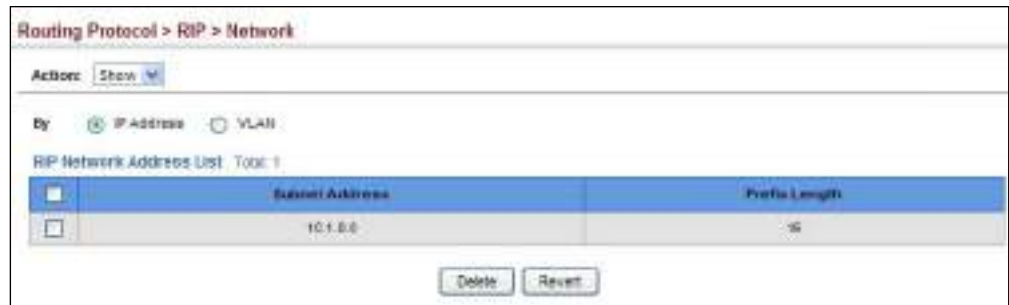
Figure 526: Showing Network Interfaces Using RIP
