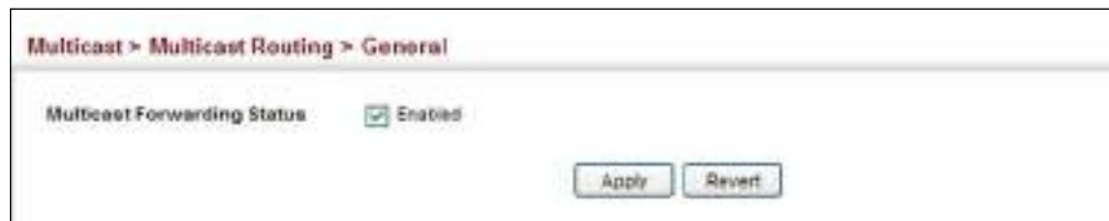
Figure 567: Enabling IPv4 Multicast Routing
