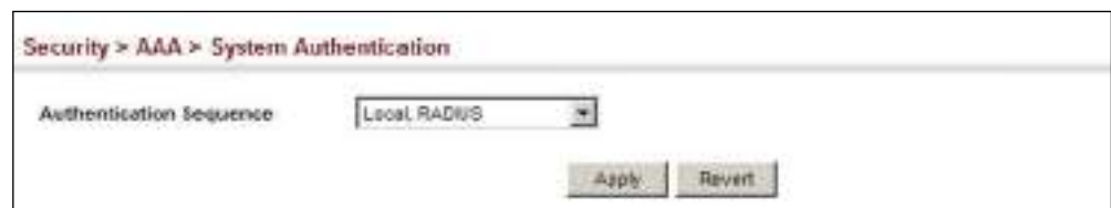
Figure 172: Configuring the Authentication Sequence
