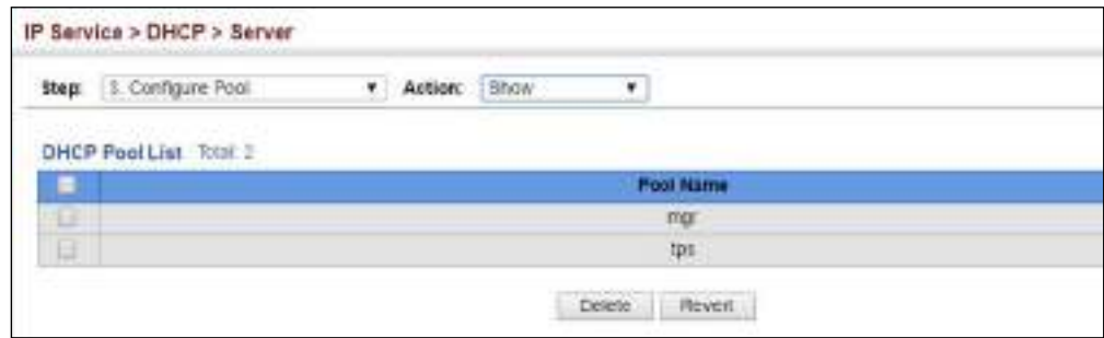
Figure 498: Showing Configured DHCP Server Address Pools
