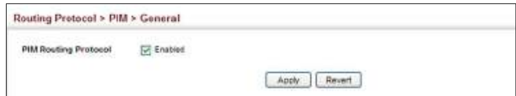
Figure 573: Enabling PIM Multicast Routing
