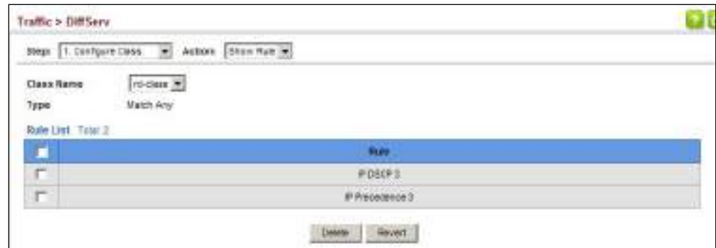
Figure 162: Showing the Rules for a Class Map
