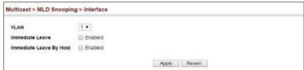
Figure 396: Configuring Immediate Leave for MLD Snooping
