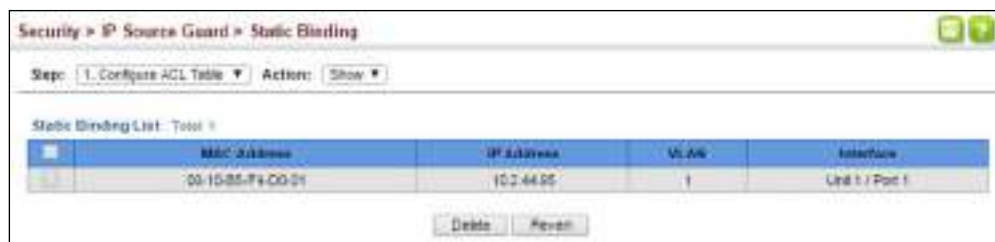
Figure 245: Displaying Static Bindings for IPv4 Source Guard
