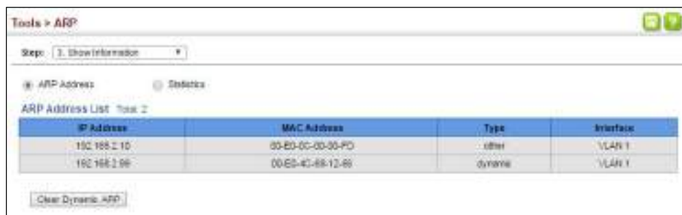
Figure 456: Displaying ARP Entries
