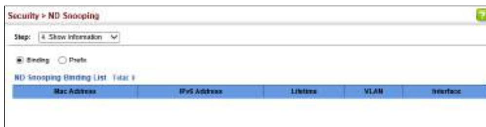
Figure 241: Displaying the Binding List for ND Snooping
