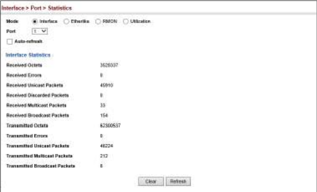
Figure 33: Showing Port Statistics (Table)
