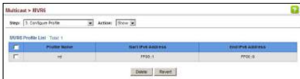
Figure 439: Displaying MVR6 Group Address Profiles
