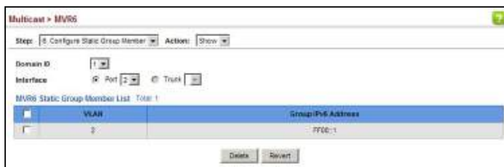
Figure 444: Showing the Static MVR6 Groups Assigned to a Port
