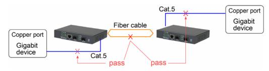
Both Gigabit devices will also detect a link fault on each Cat.5 connection, although the real fault occurs on the fiber connection exactly.
