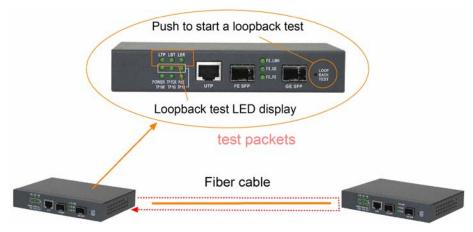
It allows installer to perform diagnostic to the fiber link during installation and check the test result displayed on the LED indicators.
