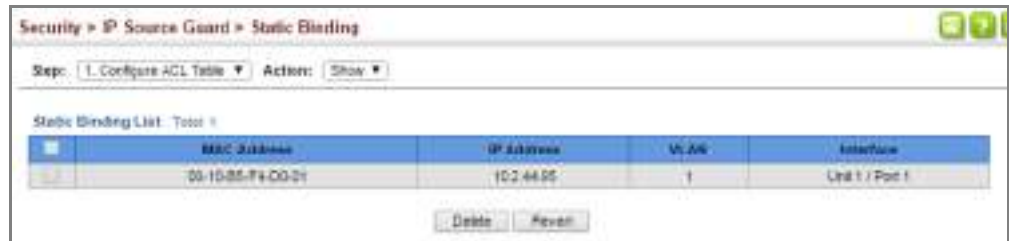
Figure 194: Displaying Static Bindings for IPv4 Source Guard
