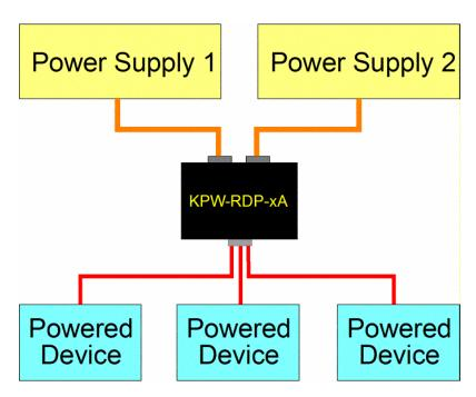
This application shows supplying power to three devices with two redundant power supplies.
