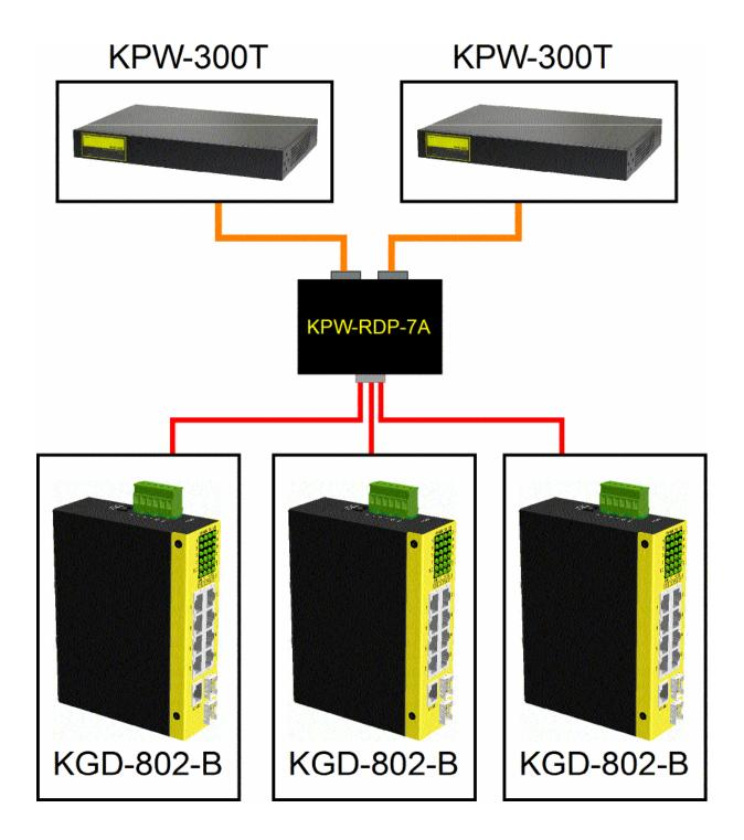
KPW-300T is 300W power supply for PoE/PoE+ applications. KGD-802-B is PoE Gigabit Ethernet switch.
