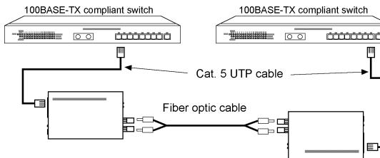
The following example illustrates a connection from a 100BASE-TX port of one hub to a 100BASE-FX port of a switch unit through a converter. A hub port is MDI-X type normally.
