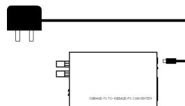
2. Connect the power adapter cable to the media converter before connecting the adapter to the AC outlet.
