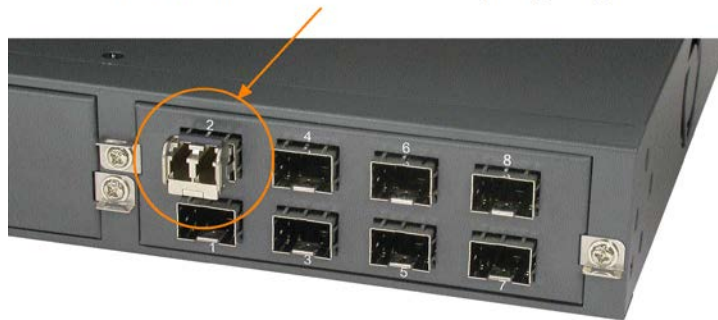
The transceiver seated properly
