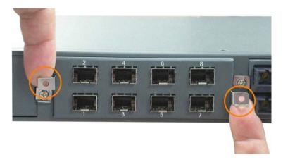
4. Remove the module from the slot.
