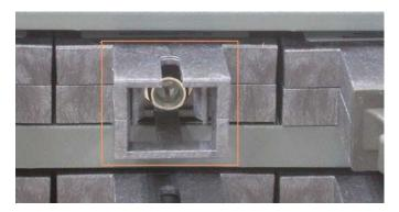
A Bi-Di port supports single fiber connection. It uses different optical wavelengths for transmission and receiving individually as figure illustrated below:
