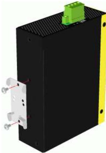
2. Attach bracket to the lower edge of the DIN rail and push the unit upward a little bit until the bracket can clamp on the upper edge of the DIN rail.
