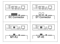
The wavelength used is 1300nm. The series also support MM (multimode) fiber cables and SM (single mode) fiber cables. The recommended MM cable is  $62.5/125\mu m$  and SM cable is  $9/125\mu m$ .
