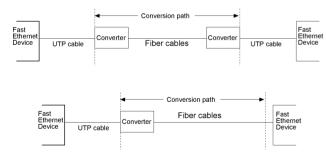
**Important rule:** When a connection is established, make sure the devices located at both ends of the path are configured and operated using the same duplex mode and the maximum distance must comply with IEEE 802.3u specifications.
