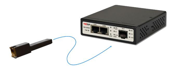
Note: The SFP Transceiver compatible to SFP slot which support 1000X/SerDes interface, please check compatibility before installation.
