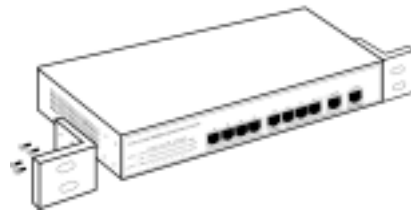
Figure 2- 2A. Attaching the mounting brackets to the Switch
