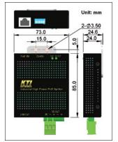
KTI Network's KPW-T2P25 is a high power PoE splitter which integrates Power over Ethernet (PoE) technology to PoE incapable network device by just using a single Cat.5 cable for both power and data transaction. The equipments such as Wireless Router, AP, Network Camera, Print server, and Media converter which connect to the PoE splitter, all devices become PoE enabled to eliminate the need of power outlets as well as cable installation and expense.
